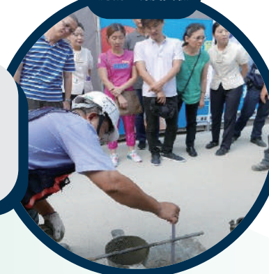
混凝土坍度實驗
